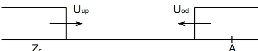
$$\begin{aligned} U_A &= U_{up} + U_{od} \Rightarrow U_{od} = U_A - U_{up} \\ I_A &= I_{up} + I_{od} = \frac{U_{up}}{Z_{c1}} - \frac{U_{od}}{Z_{c1}} \\ I_A &= \frac{U_{up}}{Z_{c1}} - \frac{U_A - U_{up}}{Z_{c1}} = \frac{2U_{up} - U_A}{Z_{c1}} \end{aligned}$$
