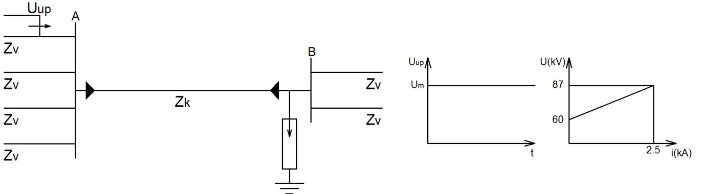
$$T = \frac{d}{v_k} = \frac{300 \text{ m}}{150 \frac{\text{m}}{\mu\text{s}}} = 2 \mu\text{s} \quad Z_{ek} = \frac{Z_v}{4} = 100 \Omega$$
