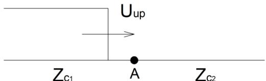
$$u + Z_{c1} i = 2U_{d1} = 2U_m \quad (1) \quad u + Z_{c2} i = 2U_{d2} \quad (3)$$
