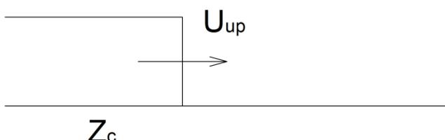
$$u = U_d + U_i \quad i = I_d + I_i = \frac{U_d}{Z_c} - \frac{U_i}{Z_c}$$
