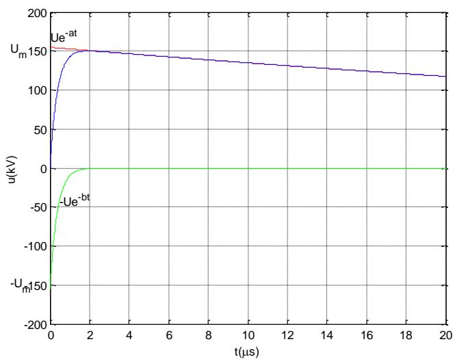
$$u(t) = \frac{U_m}{\left(\frac{a}{b}\right)^{\frac{a}{a-b}} - \left(\frac{a}{b}\right)^{\frac{b}{a-b}}} \left( e^{-at} - e^{-bt} \right)$$
