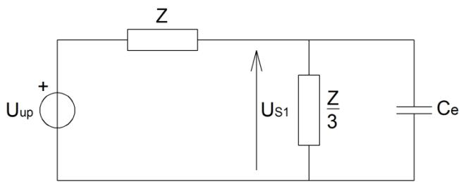
$$U_{S1}(p) = \frac{\frac{Z}{3} \frac{1}{pC}}{\frac{Z}{3} + \frac{1}{pC}} \frac{2U_{up}(p)}{Z + \frac{Z}{3} \frac{1}{pC}} = \frac{\frac{Z}{3} \frac{1}{pC}}{\frac{3 + ZpC}{3pC}} \frac{2U_{up}(p)}{Z + \frac{Z}{3 + ZpC}}$$
