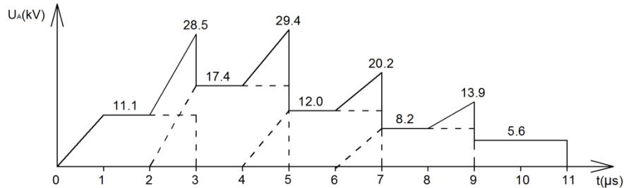
$$U_{Amax} = 29,4 \text{ kV} < U_{100\%} = 43 \text{ kV}$$
