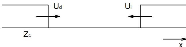
$$U = U_d + U_i \quad I = I_d + I_i = \frac{U_d}{Z_c} - \frac{U_i}{Z_c}$$
