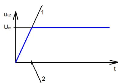
$$u_{up}(t) = \underbrace{ath(t)}_1 - \underbrace{a(t - T_c)h(t - T_c)}_2$$
