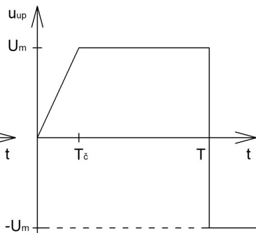
$$u_{up}(t) = ath(t) - a(t - T_c)h(t - T_c) - U_mh(t - T); \quad a = \frac{U_m}{T_c}$$
