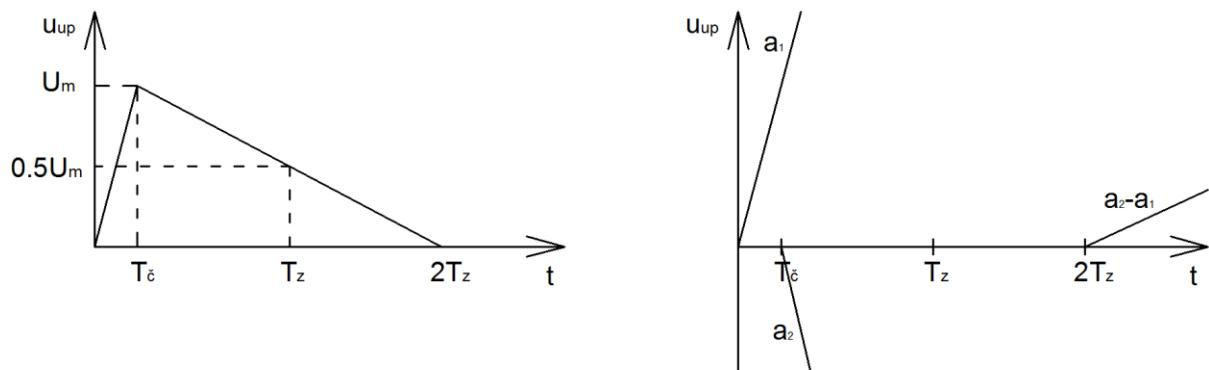
$$u_{up}(t) = a_1 t h(t) - a_2 (t - T_c) h(t - T_c) + (a_2 - a_1)(t - 2T_z) h(t - 2T_z) \quad T_z \gg T_c$$
