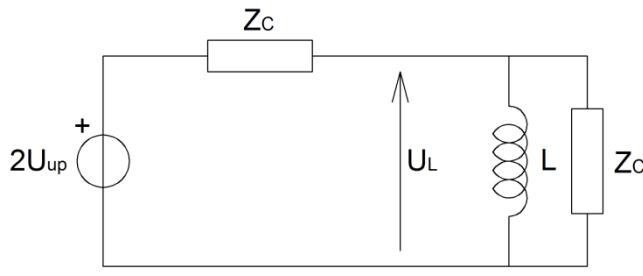
$$U_L(p) = \frac{Z_c p L}{Z_c + pL} \frac{2U_{up}(p)}{Z_c + \frac{Z_c p L}{Z_c + pL}} = \frac{pL}{Z_c + pL} \frac{2U_{up}(p)}{\frac{Z_c + pL}{Z_c} + pL}$$
