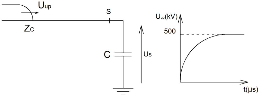
$$u_{up}(t) = U_m(1 - e^{-bt}) \quad b = \frac{\ln 7}{0,6 \cdot T_c} = 2,7027 \frac{1}{\mu\text{s}}$$
